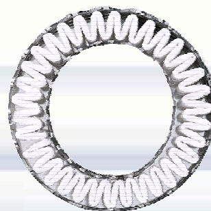
Cross-sectional diagram of FLUIDAIR element with pleated media
